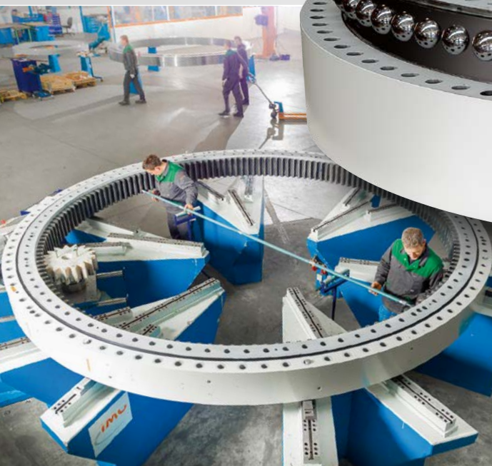
3 MW-class blade bearing, ► hydraulic pitch
