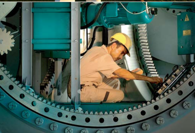
◀ 2 MW-class blade bearing, electric pitch / internal gears
